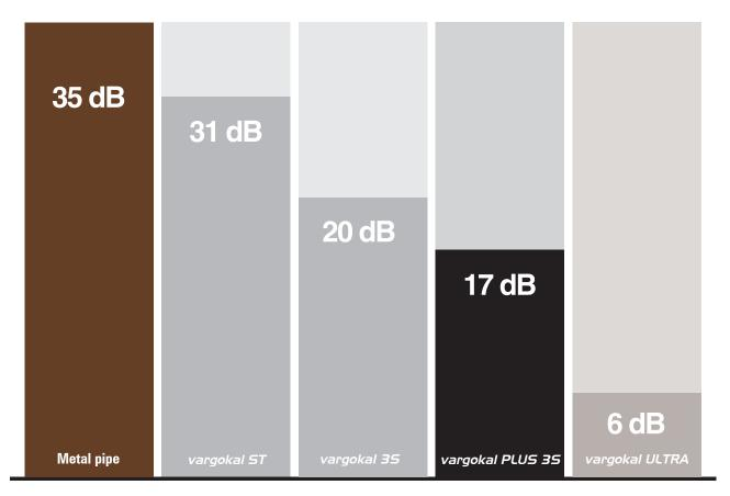
The table shows the noise level at a flow rate of 2 liters of water per second.
