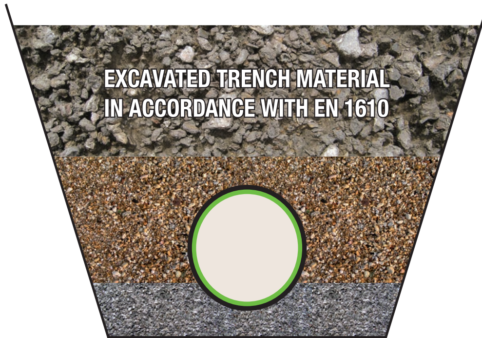
The picture shows a properly installed vargokor pipe
