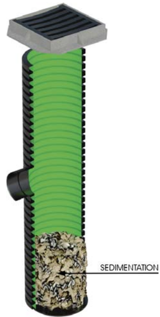
Cross-section of catchpit
