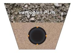
During installation, the rules on safety at work should be followed. The trench must be properly drained, and all joints should be left free until a leak test is performed.
