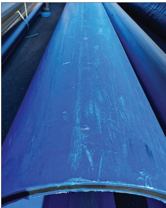
Visible line and point damage on the pipe surface
