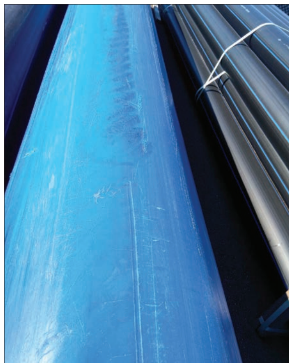
Visible line and point damage on the pipe surface
